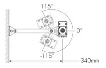
WAM18 - Adjustable Extended Arm Mounting 457 mm
